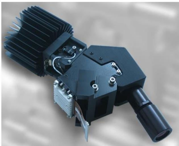
Lumaxis designs high-performance Projection Engines for manufacturers of 3D optical metrology solutions.
