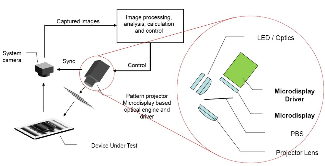
The projector projects an area that is usually smaller than the DUT. The projected area is often called Field of View (FoV), and will have certain brightness and relative contrast ratio requirements. SLP offers the best potential for achieving design goals such as speed, accuracy and cost.
